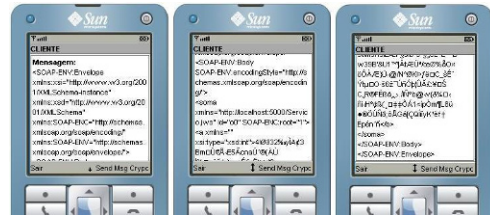
Figure 9 – Sample of Encrypted Message in Mobile Device
