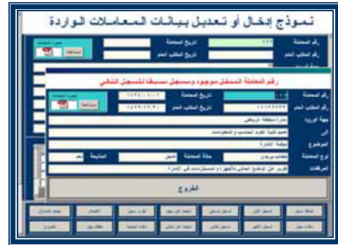
Figure ( 3 ) Shows the form displaying the information of the stored record when entering a duplicate document ID number which belongs to a previously stored document record since the document ID number field is the primary key.
