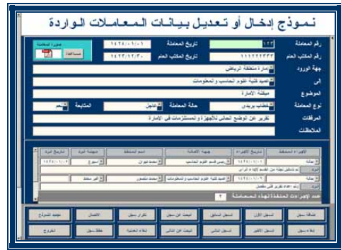
Figure ( 2 ) Shows the main data entry form for the incoming documents after passing through the authorization screen. The green field indicates the primary field. The user may use the command keys on the bottom of the form to manipulate the data or/and add new records, In addition to the search keys to search through the previously stored faculty records.
