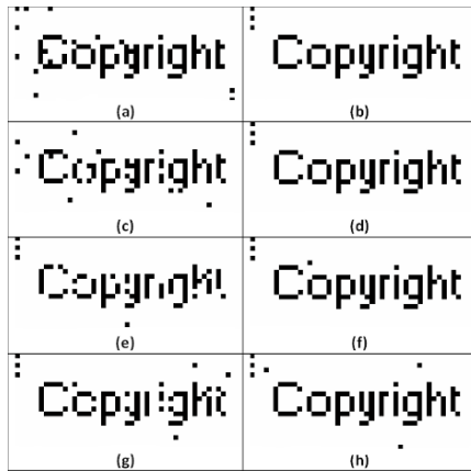
Fig. 8. Recovered watermark after, (a) Shrink attack Hsu (b) Shrink attack Koch (c) JPEG 4 attack Hsu (d) JPEG 4 attack Koch (e) Poisson Noise attack Benham (f) Poisson Noise attack Koch (g) Median attack Benham (h) Median attack Koch, watermarked Lena image
